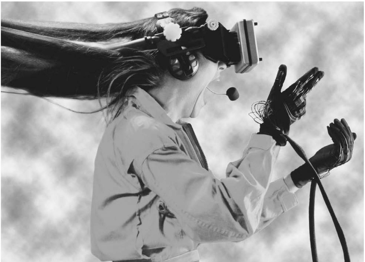
A NASA researcher wearing Virtual Interactive Environment Workstation (VIEW) apparatus. Created in the late twentieth century, VIEW manipulated sensory input to transport a person to another reality in which they could manipulate objects. NASA/PHOTO RESEARCHERS, INC.
