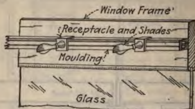
FIG. 105.—Show-window wiring in molding.
