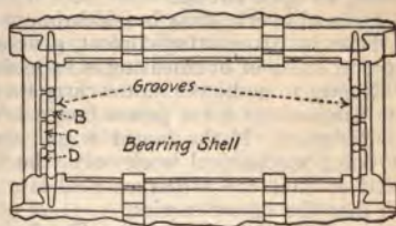
FIG. 72.—Grooves to prevent oil leakage.
