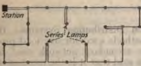
FIG. 112.—Open loop series circuit.
