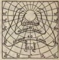
FIG. 21.—Typical photometric curves of lamps with "extensive" reflectors.
