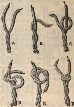
FIG. 9.—Method of tying supporting knot in flexible cord. (See Par. 9 for description.)
