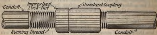
FIG. 151.—Showing lock-nut sawed from coupling.
