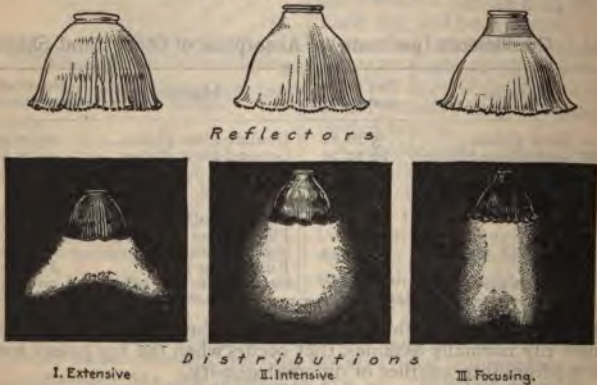
FIG. 20.—Typical prismatic glass reflectors.
