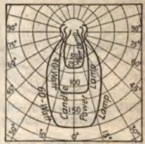
FIG. 23.—Typical photometric curves of lamps with "focussing" reflectors.
