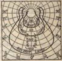
FIG. 22.—Typical photometric curves of lamps with "intensive" reflectors.
