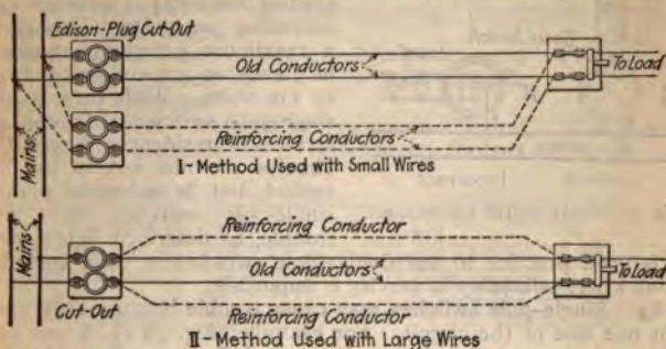
FIG. 35.—Methods of reinforcing conductors.
