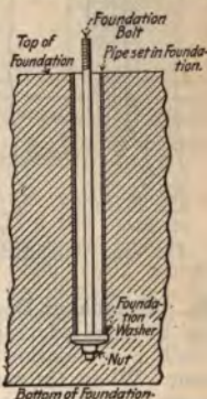
FIG. 112.—Bolt set in foundation.
