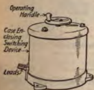
FIG. 89.—Enclosed starter for a phase-wound motor.
