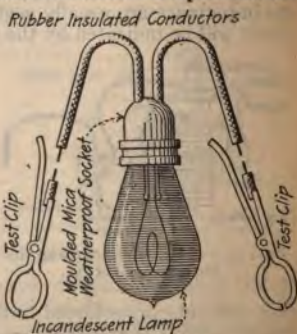
FIG. 48.—A practical test-lamp outfit.
