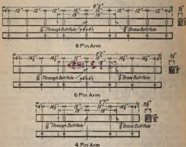
FIG. 40.—Cross-arm dimensions recommended by the N. E. L. A.
