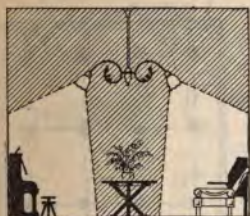
FIG. 37.—Effect of hanging residence lamps at an angle.
