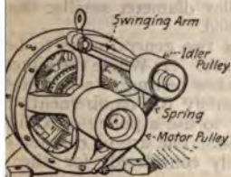
FIG. 128.—Idler pulley attachment to increase arc of contact.
