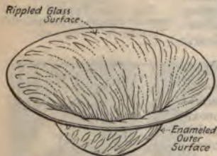
FIG. 24.—Silvered reflector for indirect lighting.
