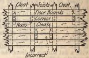
FIG. 272.—Methods of locating cleats to support floor boards that have been removed.
