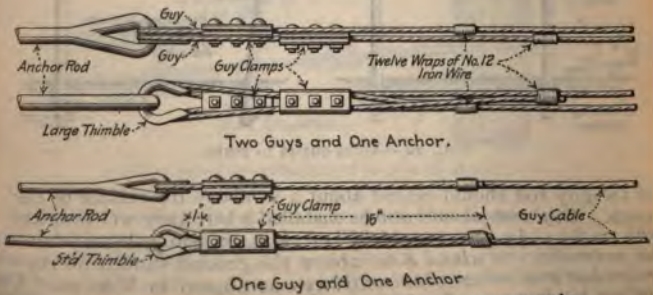
FIG. 25.—Methods of making up guys on guy rods.
