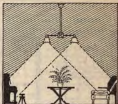
FIG. 38.—Effect of hanging residence lamps vertically.
