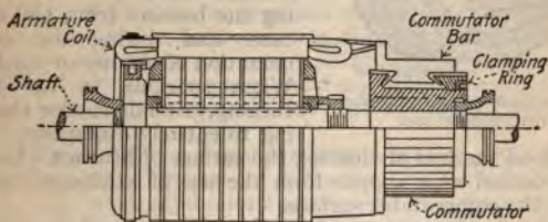
FIG. 39.—Section of direct-current motor armature.
