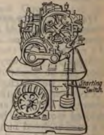
FIG. 127.—Countershaft geared to motor.
