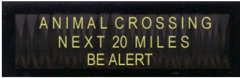
Figure 29. Sign Treatment 3 – Dynamic Message Sign.
